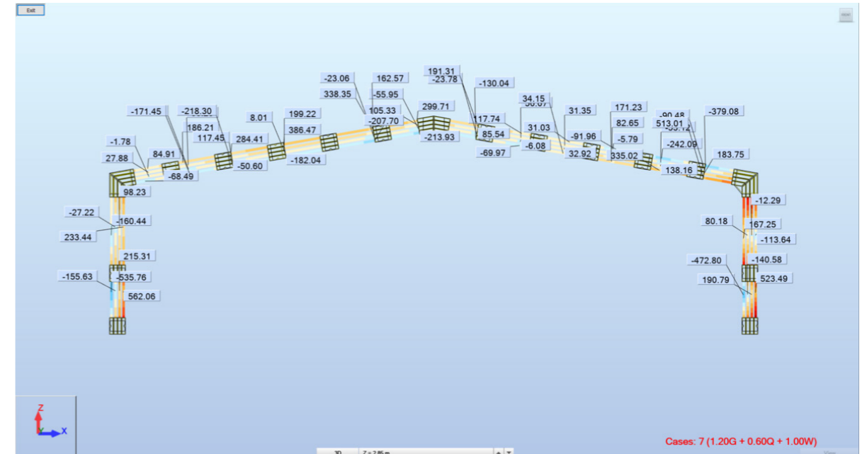
Finite element analysis of version 1 member stresses (N/mm 2 ) with a load combination: 1.20G + 0.60Q + 1.00W.
