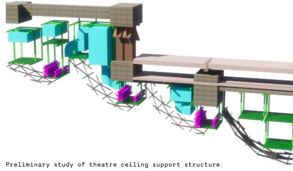
3D view of proposed ladder frame and cladding support structure.
