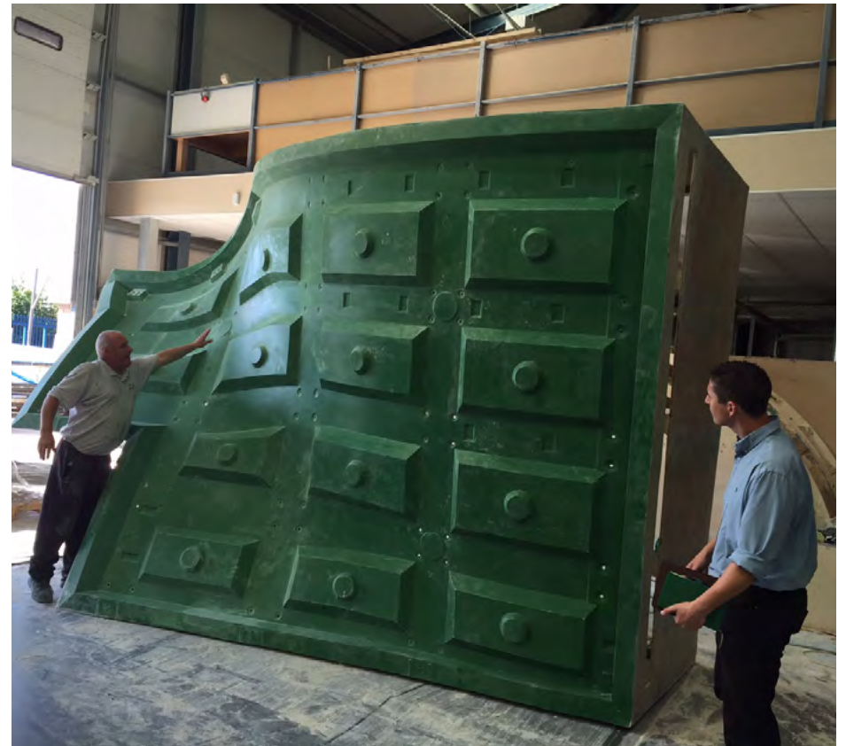
Below: Complex mould for a tunnel lining element, milled directly from the model by CNC machine.
